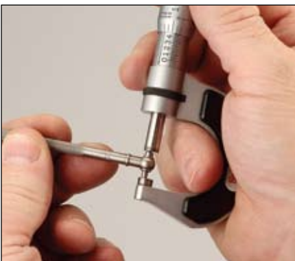
After establishing hole size with a telescoping gage, actual size is determined by measuring over the contacts with an outside micrometer.
