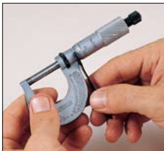
Illustrated: Adjusting for zero reading.
