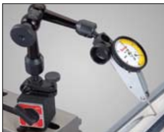
709B Dial Test Indicator attached to a 660 Magnetic Base Indicator Holder in an application to check for roundness.
