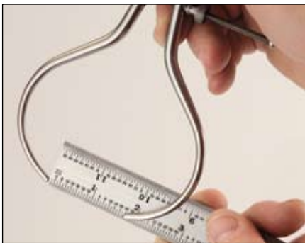
Pre-setting outside calipers to a rule for a transfer measurement.
