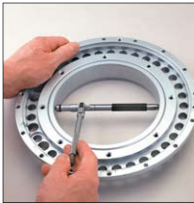
Checking inside diameter of a deep hole with an inside micrometer. Convenient handle is attached to the center of the micrometer.
