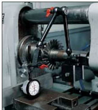
631 Back Plunger Dial Indicator attached to No. 657-1 Magnetic Base Universal Indicator Holder.
