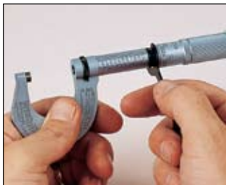
Illustrated: Adjusting spindle play.
