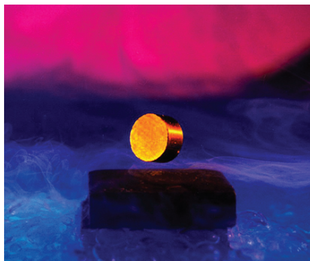
Figure TF3-1: The Meissner effect, or strong diamagnetism, seen between a high-temperature superconductor and a rare earth magnet. (Courtesy of Pacific Northwest National Laboratory.)
