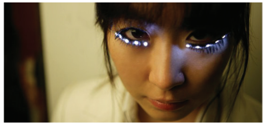
Figure TF5-4: LED eyelashes can be worn in many colors, and can be made to turn on or off with a tip of the head. (Credit: Soomi Park.)
