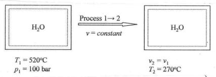
Since the process occurs at constant volume,  $v_2 = v_1$ . State 1 is fixed by the given property values,  $T_1 = 520$  °C and  $p_1 = 100$  bar. From Table A-4,  $v_1 = 0.03394$  m<sup>3</sup>/kg.
